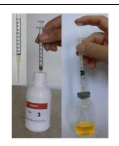
**3**. Fill the syringe with Reagent 3 to the highest mark (1 ml). Add Reagent 3 by drops until the color become light yellow. Swirl to mix after each drop.
