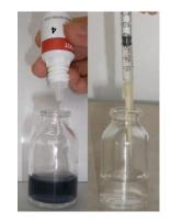
**4**. Add 1 drops of Reagent 4. Water turns blue or violet. Drop Reagent 3 until colorless end point. Note the used volume of the Reagent 3.
